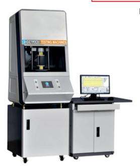
The ZGT MV 3000AU Mooney Viscometer measures the viscosity, scorch and stress relaxation of raw rubber or compounded rubber. It is used for determining the quality of rubber processing characteristics. By knowing the properties of Mooney viscosity and stress relaxation, the molecular weight and distribution range can be determined. The ZGT MV 3000AU is equipped with PC based dedicated software, accurate temperature control system and automatic calibration device.
